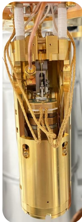
Right: mK scanning probe microscopy with laser optical interferometer feedback.
