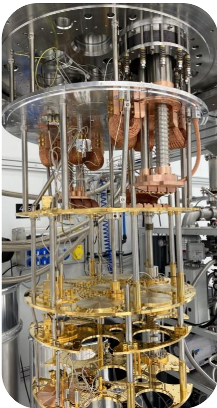
Right: mK scanning probe microscopy with laser optical interferometer feedback.
